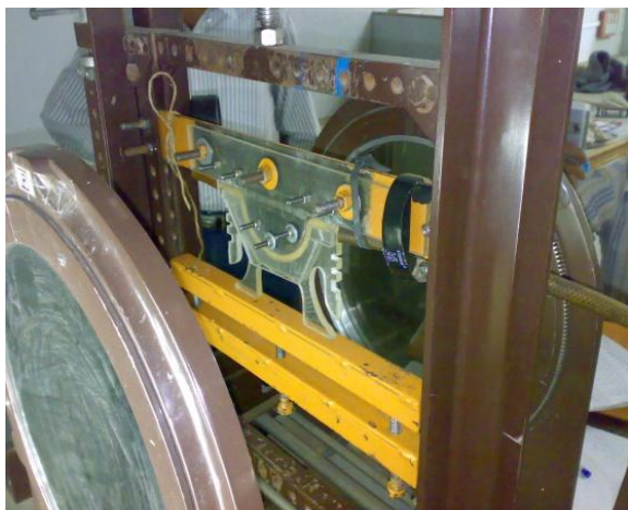
Fig. 2(b). Experimental set up on polariscope
